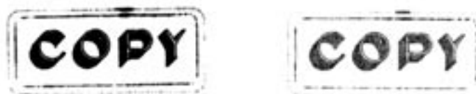
FIG. 5—Test prints of questioned pre-inked stamp showing first and second test impressions using a black ink stamp pad.
